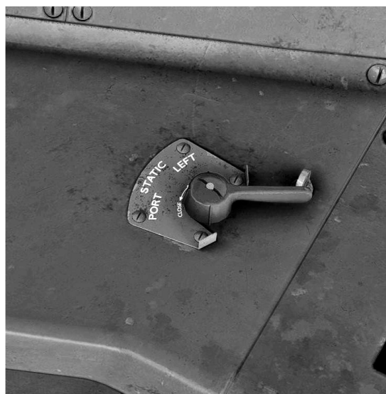
Installation of the static valve of the right pilot.
