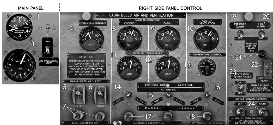
Control panel of the de-pressurization, heating and ventilation
