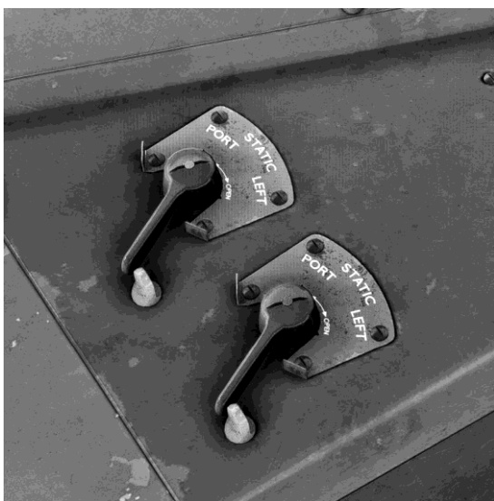
Installation of dynamics and statics valves of the left pilot.
