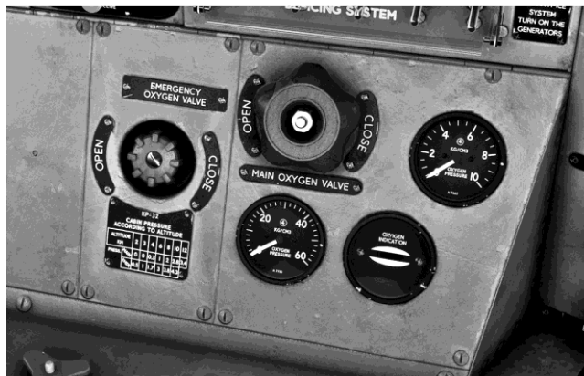
Installation of the oxygen system control panel on the right pilot's panel
