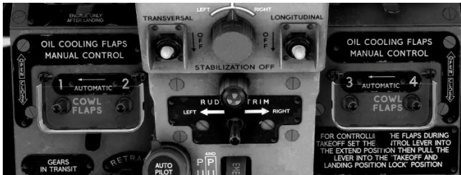
Cowl flaps control on the central console.
